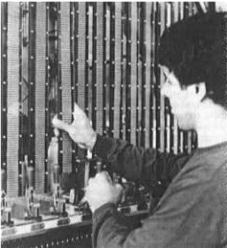
Figure 9. Slug Rivet Feed System
