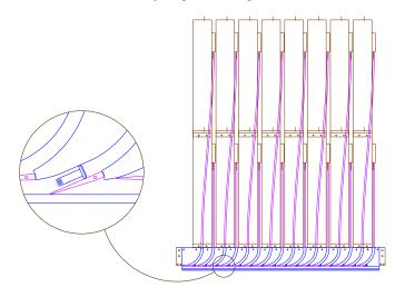
almost any size or shape in an end-to-end configuration. Each magazine holds its own passive **escapement** within the magazine. Headed fasteners are escaped with a one-moving-part escapement, which works with all fasteners of a given shank diameter (Figure 6). Slug rivets are escaped with a one-moving-part escapement which is diameter specific but length independent (Figure 7).
