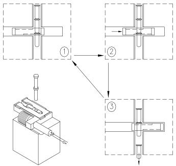
Figure 6. Headed Fastener Escapement
