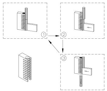
Figure 7. Slug Rivet Escapement
