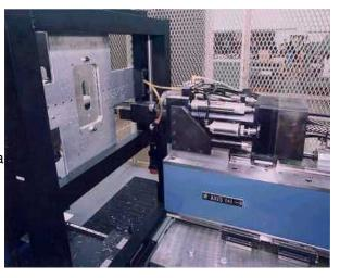
The operator interface, including two button panels, the Fanuc 15-MB CNC monitor and the maintenance PC a mounted in the operator console. Near the operator console is a small cabinet outfitted with fastener feed equipment: five drop tubes, a two-slot fastener magazine rack, and 3/16 automatic collar escapement. The entire test bench work area has a plywood raised floor to place the test bench tools at a comfortable working height.
