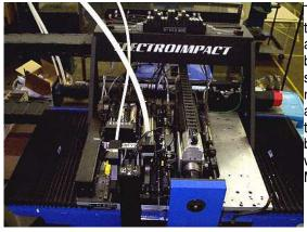
The shuttle table is located above the Z clamp table. The shuttle table is a precision ground aluminum plate. Below the shuttle table are linear bearings that allow the table to move to the several tool positions. Inset into the table are round and diamond dowel pins for tool alignment, and steel inserts into which screw the individual tool mounting bolts. The shuttle table was aligned by Electroimpact personnel when the Test Bench was installed. No alignment should be required by MDA personnel.
