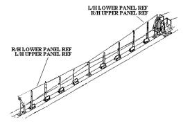
Note that the HH550 contains features in the gun which are specific to the skin side and the stringer side. Four lifts carrying EMRs were provided. There are two lifts which are always on the skin side of the wing panels and two lifts which are always on the stringer side. Note that the lifts run on tracks and there is adequate space for a parking zone at each end of the cell.
