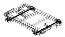
Figure 3. Anti-sway columns mounted on lift base.
