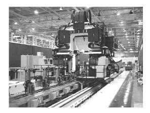
Figure 7: Spar Loaded in Fixture
