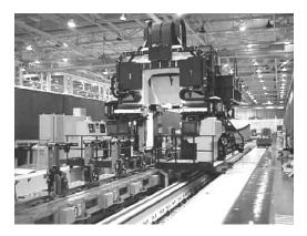
Figure 2: Clamp Table with Process Tools
