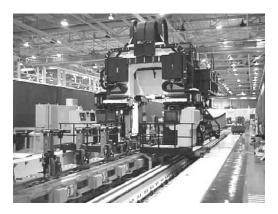
Figure 6: Loading Spar into Fixture
