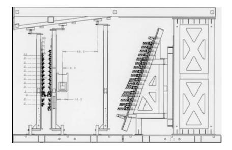
Figure 13: String side head clears the rotating support. Rotating supports provide a 48" wide workbay.
