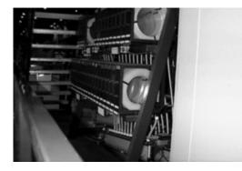
Figure 9: Cartridge fastener feed system
