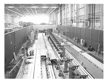
Figure 7: Spar Loaded in Fixture
