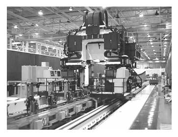
Figure 1: E5000 Machine with Redundant Operator Stations
