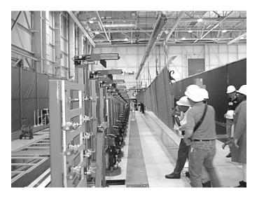
Figure 6: Loading Spar into Fixture
