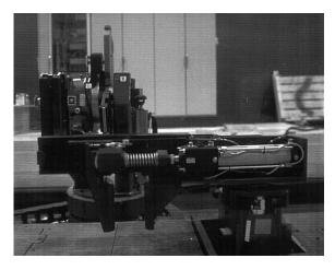
Figure 9: Upper Index Assembly with Post Fully Down
