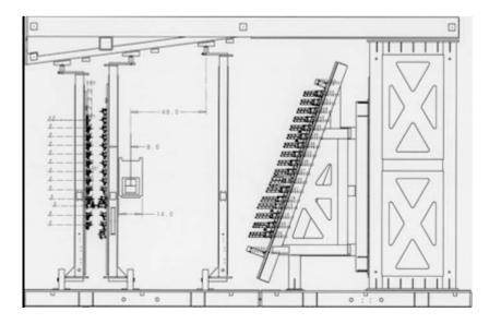
Figure 13: String side head clears the rotating support. Rotating supports provide a 48" wide workbay.
