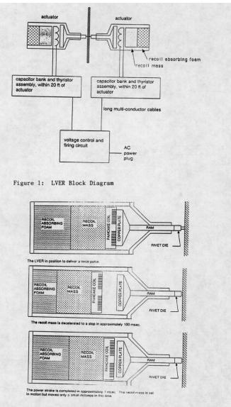
Figure 2: Operating Sequence of the LVER Recoil Control System
