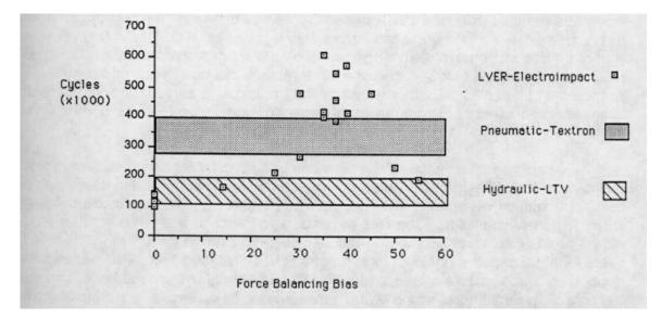
Figure 7: Effect of Force Balancing Bias on fatigue life for 7050 fatigue life for 7050 Briles countersunk rivets in .142" stack up. Test run at 24 ksi maximum stress with a .05 load ratio.
