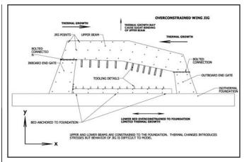
Figure 3. Thermally overconstrained jig
