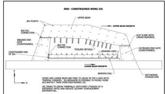
Figure 4. End-constrained wing jig
