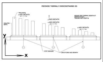
Figure 2. Simplified illustration of a piecewise thermally overconstrained jig
