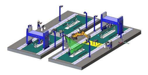
Figure 8 Conceptual AFP Cell for frames or small spars
