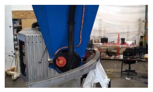
Figure 5 – Electroimpact seven axis AFP machine with swing-through head
