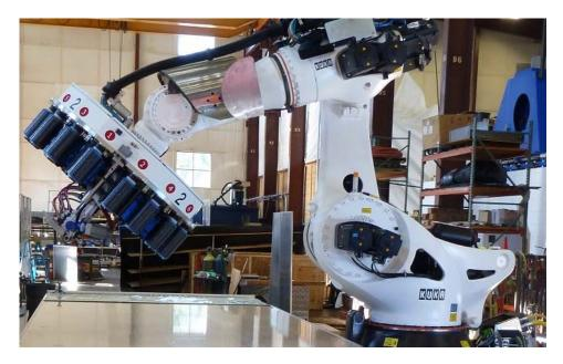
Figure 9. Robot with non-continuous axis 6. Stainless steel shroud keeps the conduit from entangling with the robot.
