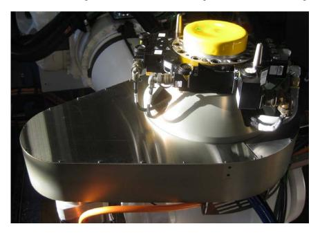
Figure 5. Complete Electroimpact designed axis 6 assembly.
