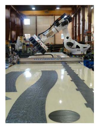
Figure 12. Typical flat charges on the vacuum table.
