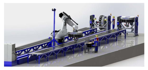
Figure 14. Robotic AFP stringer charge cell with two vacuum tables, ultrasonic cutting head, head change stands, and laser projection.
