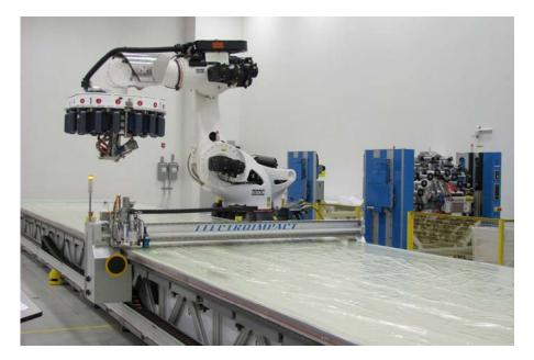
Figure 11. Robotic AFP cell with vacuum table, ultrasonic cutting gantry, 2 AFP heads (1/4" and  $\frac{1}{2}$ "), and head changing stands.
