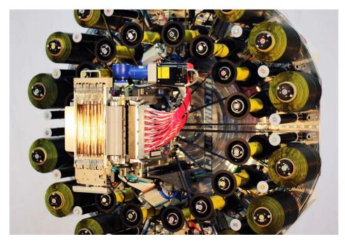
Figure 3. Modular Automated Fiber Placement (AFP) head
