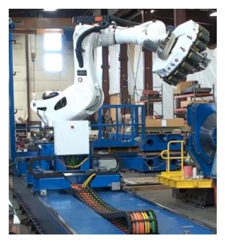
Figure 10. Fiber placement robot with axis 6 retrofit, rotators, and dual linear axes under the robot base.
