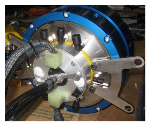
Figure 7. Pneumatic rotary union with power and signal slip-rings.
