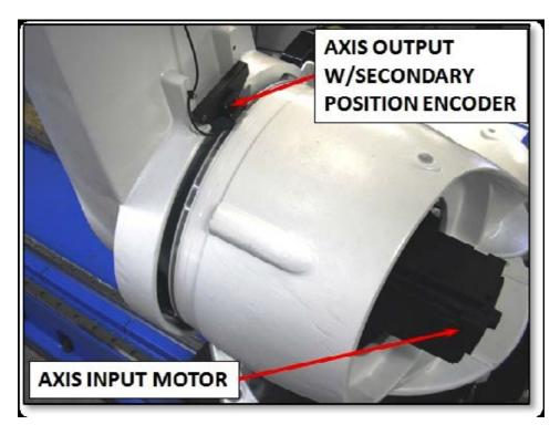
Figure 1. Industrial robot axis with secondary feedback installed.
