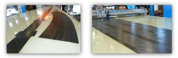
Figure 3: Steered Fiber and Neat Net Shape Layups.
