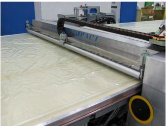
Figure 6: Rear view of Ultrasonic Cutting Gantry showing backing film pickup mechanism.
