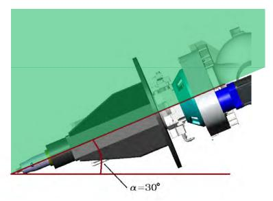
Figure 15: Rendering of High Clearance Ultrasonic Cutting Head at 30° from horizontal. Operating range shown in green.
