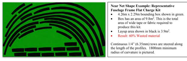
Figure 2: Near Net Shape Layup Efficiency Calculation.
