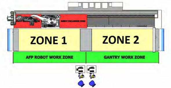
Figure 4: Work cell divided into two zones.
