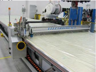
Figure 5: Front view of Ultrasonic Cutting Gantry showing main process head.
