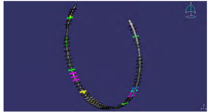
Figure 1. 777 – Buttsplice Components (splice plates, shear ties, stringer splices)
