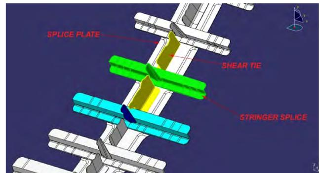
Figure 2. 777 – Buttsplice Components (Detail)
