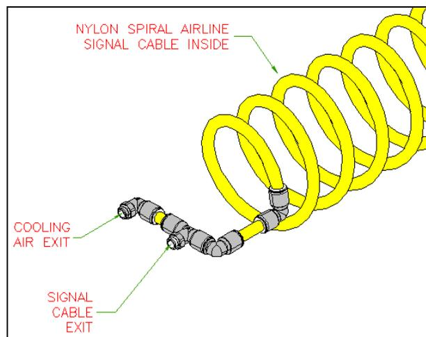
**Figure 4 – Air-Signal Segment (Actuator end)**
