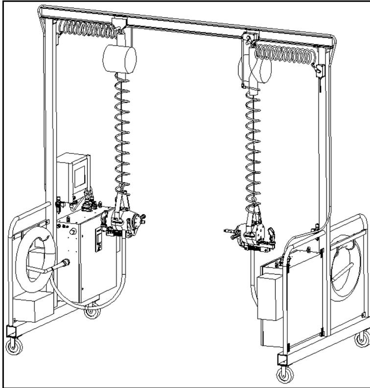
**Figure 1 - HH-553 Riveting System**
