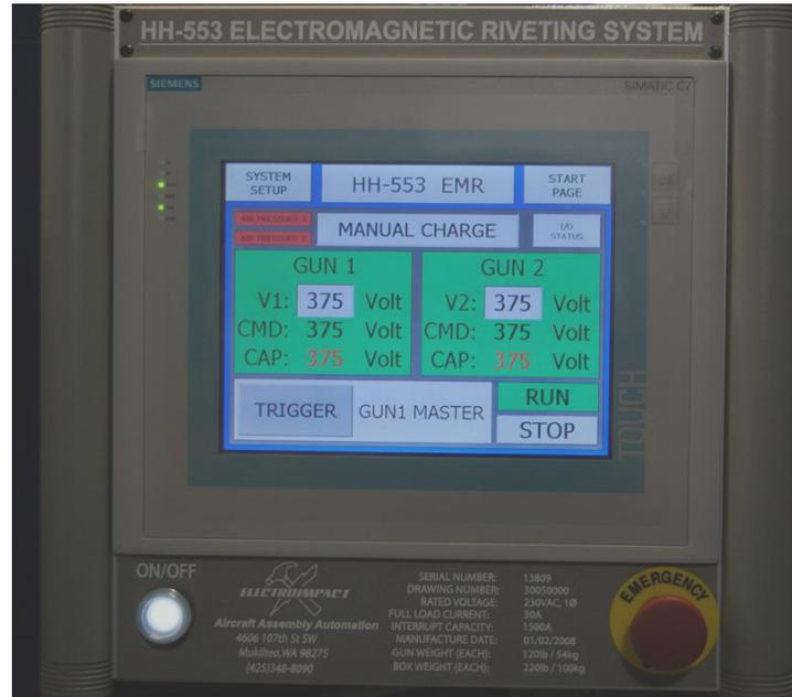
Figure 6 - Siemens Touchscreen PLC
