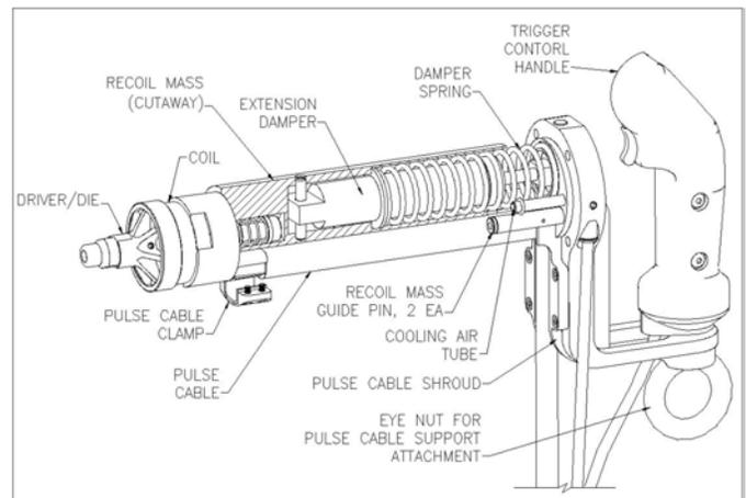
Figure 2. HH54 cutaway view of damping components.
