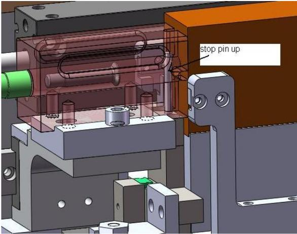
Figure 8 - Stop Pin extended
