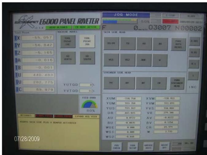
Figure 17: CNC display in Jog mode.
