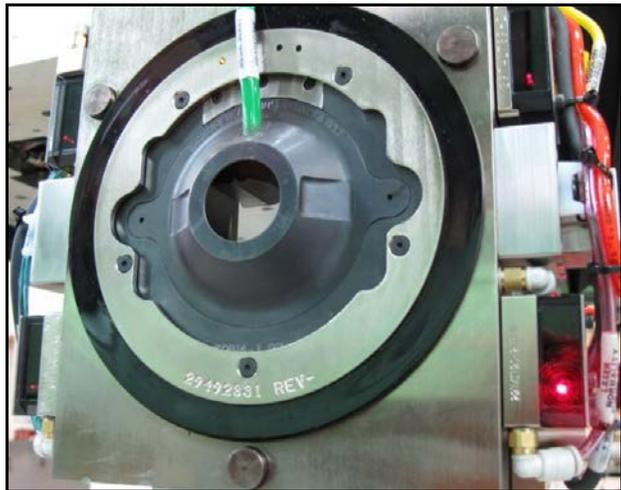
**Figure 14: Front of clamping foot with laser normality sensor array on the sides. Ring load cell is mounted in a pocket behind clamp pad at center.**
