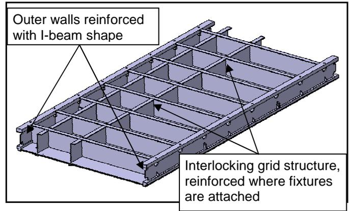
Figure 10. Underside of monolithic bed.
