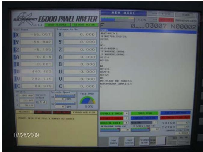
Figure 16: CNC display in Memory mode.
