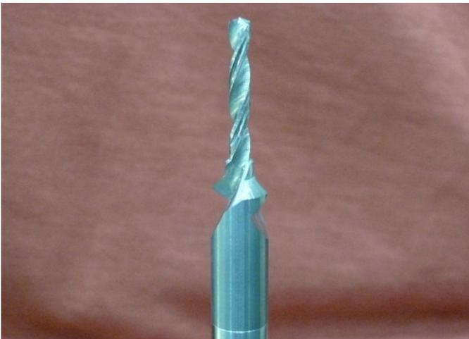
Figure 3. Carbide Drill & Countersink
