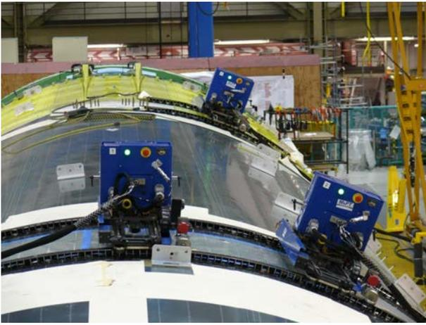
Figure 1. Flex Track Drilling Machines on 777 Fuselage
