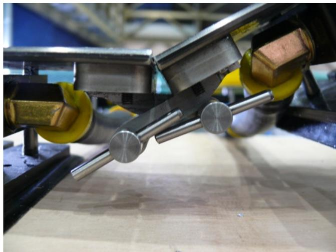
Figure 6. Quick Change Track Splice
