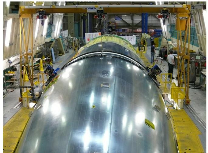
Figure 5. Gantry Handling System
