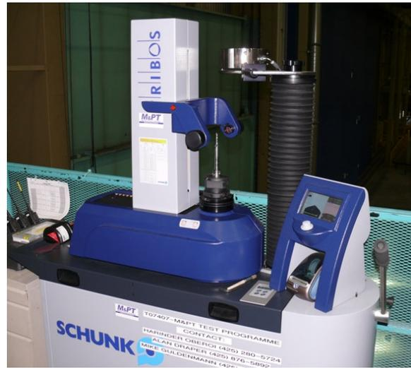
Figure 4. Tool Presetter
