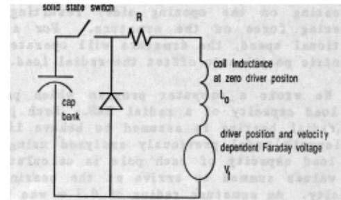
Figure 2 Capacitor Discharge Circuit
