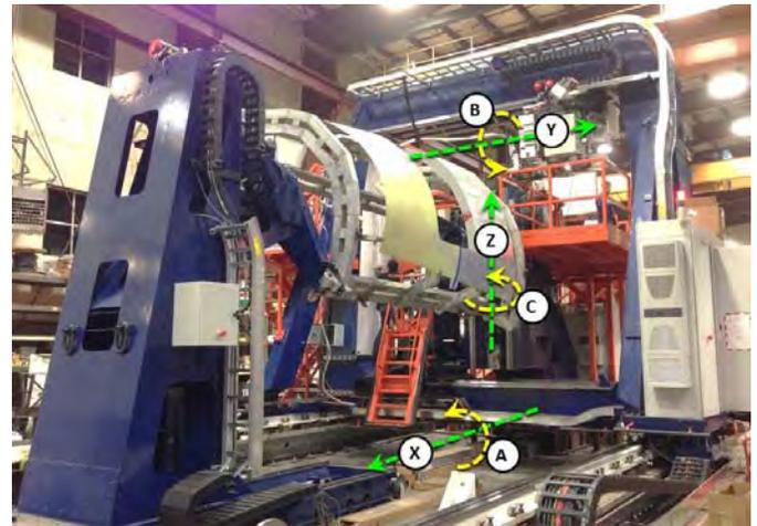
*Figure 1. Overall machine structure and axis orientations*
