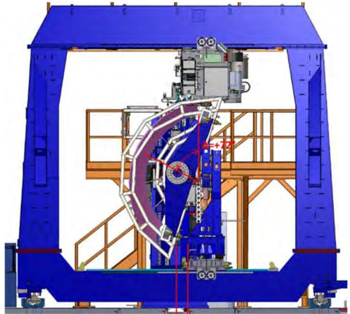
*Figure 4. E7000 machine accessing the edge of a panel that spans 144° of curvature*
