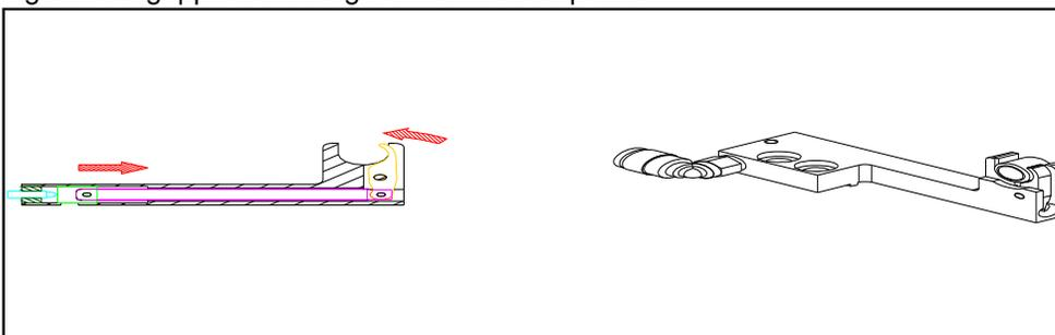
Figure 15: gripper fingers gripping collar
