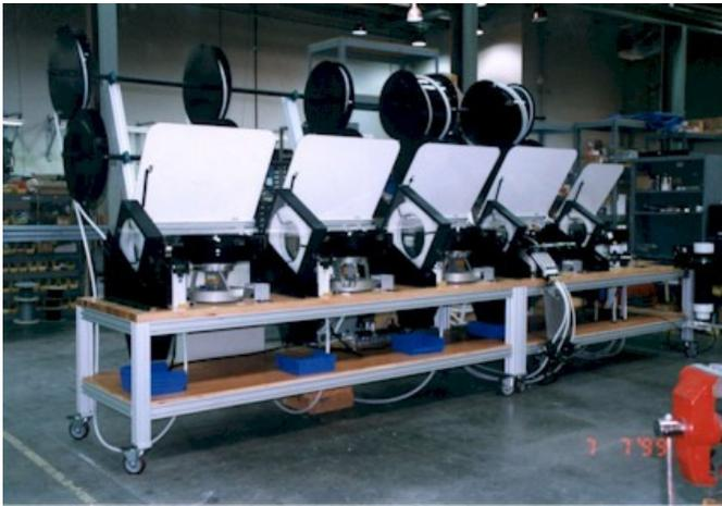
Figure 5. A five bowl CFS for 10 fastener types, 72 fasteners in total
