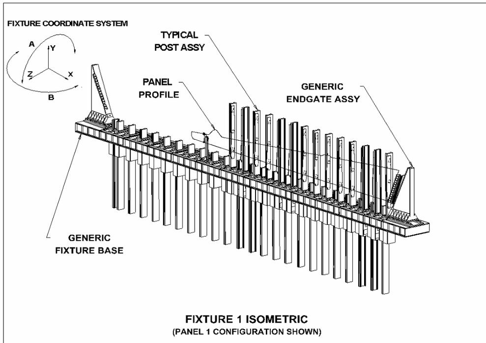
Figure 2: Flexible "Popping Post" Fixture
