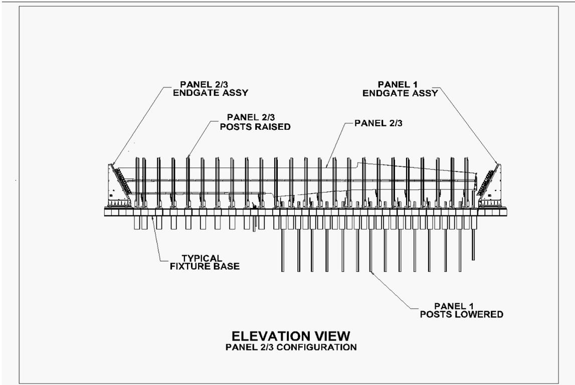
**Figure 4: Side View in Panel 2/3 Configuration**
