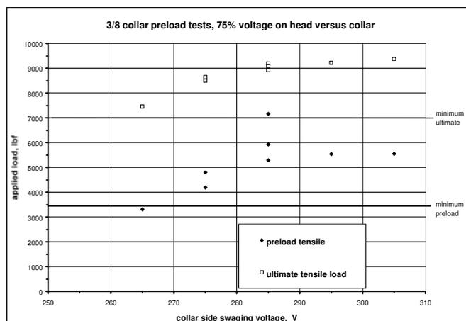
Figure 8. 3/8 Collar Pre-load Tests
