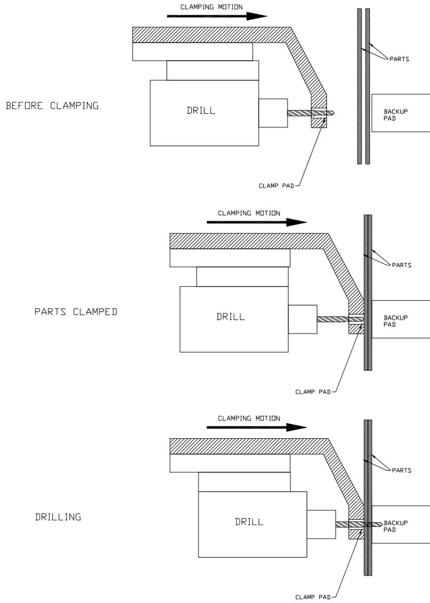
FIGURE 1 – DRILLING PROCESS
