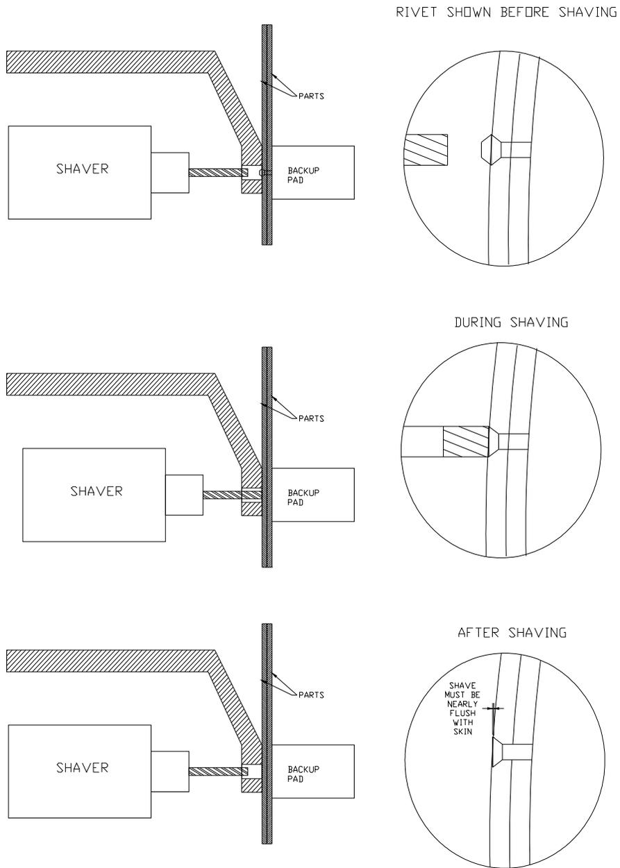
FIGURE 5 – RIVET SHAVING PROCESS
