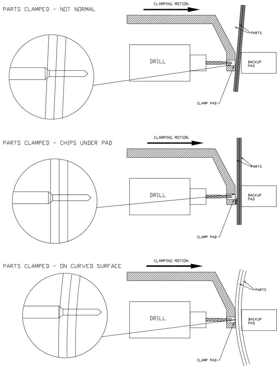
FIGURE 3 – CAUSES OF DEPTH ERROR
