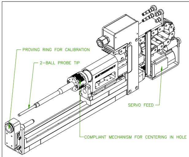
Figure 6: Hole Probe
