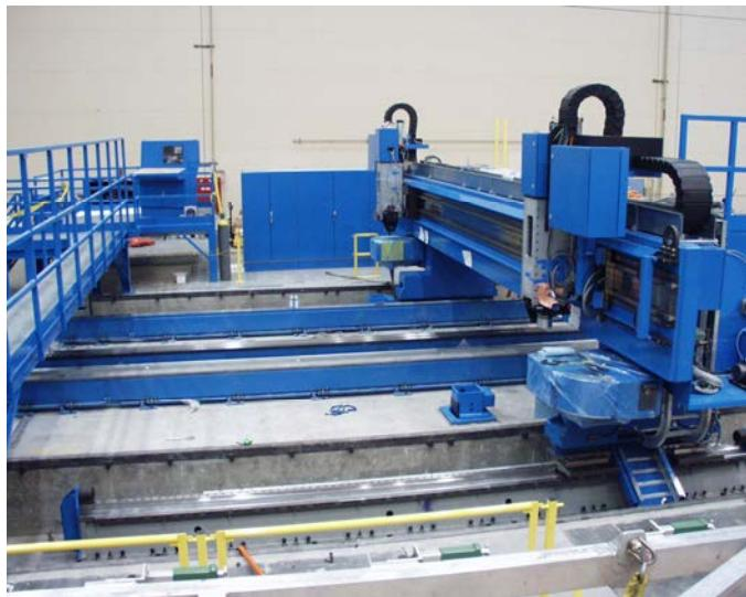
**Figure 1: Gantry Drill Machine
