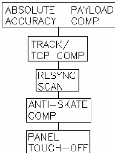
compensating for this deflection in an equal and opposite manner. Compensation motion is triggered as panel contact is established. The result has been the reduction of skating by 80-100% in all positions regardless of panel to nose tip friction, robot orientation, and clamp load. Calculations are made on the fly and are completely transparent to the operator and programmer.
