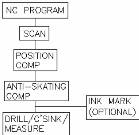
The system process begins with the off-line generation of NC programs. The Cell Control executes NC programs that are generated with custom software built around IGRIP, a robotics simulation and off line programming software package available from Delmia Corp. The TEF is then loaded into the holding fixture.
