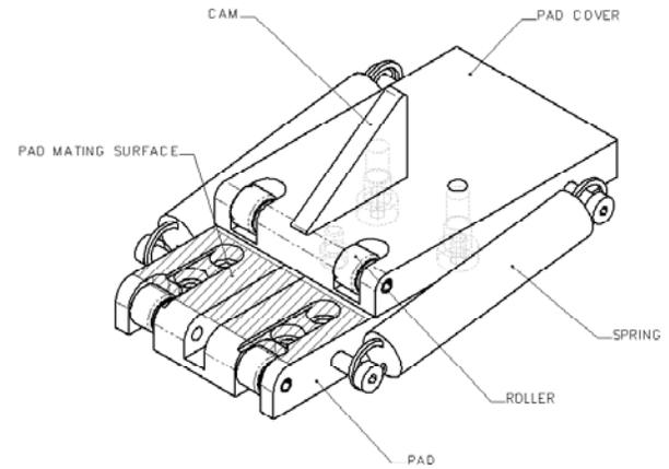
**Figure 10 - Machine Pad**
