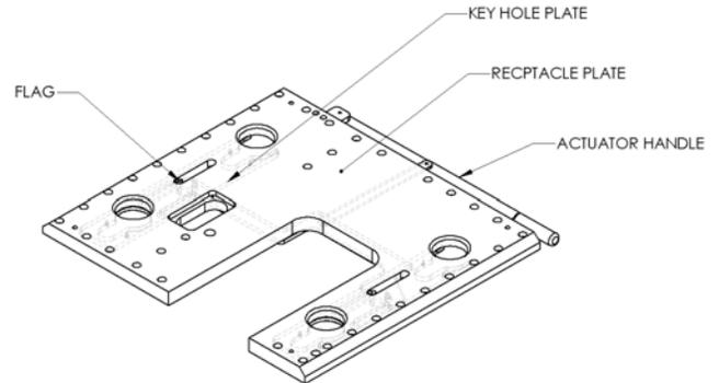
**Figure 8 - Transporter receptacle plate on GRAWDE**
