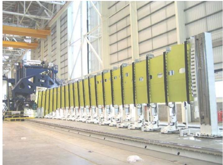
Figure 1 Two tower riveting machine
