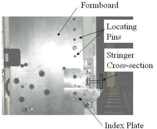
Figure 3: Prototype A380 pegboard ("formboard") and one index-plate
