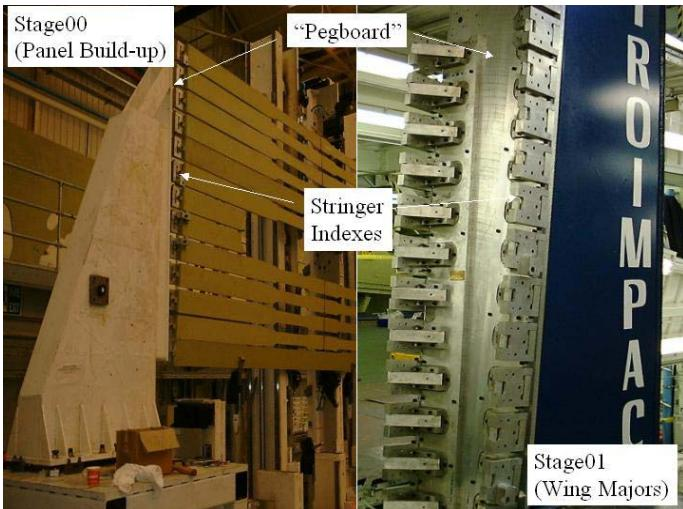
Figure 2:Determinate Assembly on A340-600 test-panel tooling modifications
