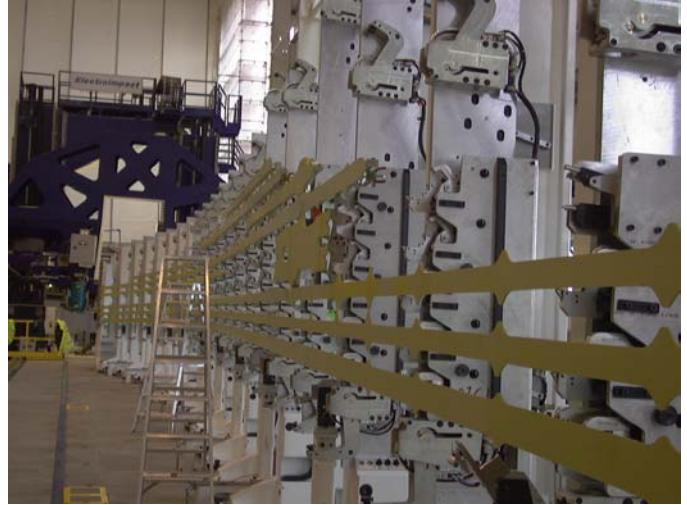
*Figure 6: Completed A380 panel-build fixture with stringers partially loaded*
