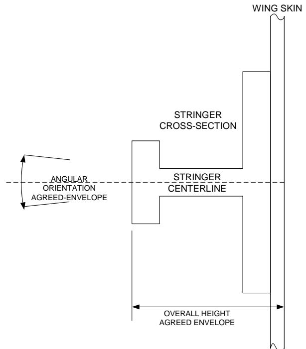
Figure 4: Typical envelopes of allowable stringer cross-section changes, agreed between design and tooling
