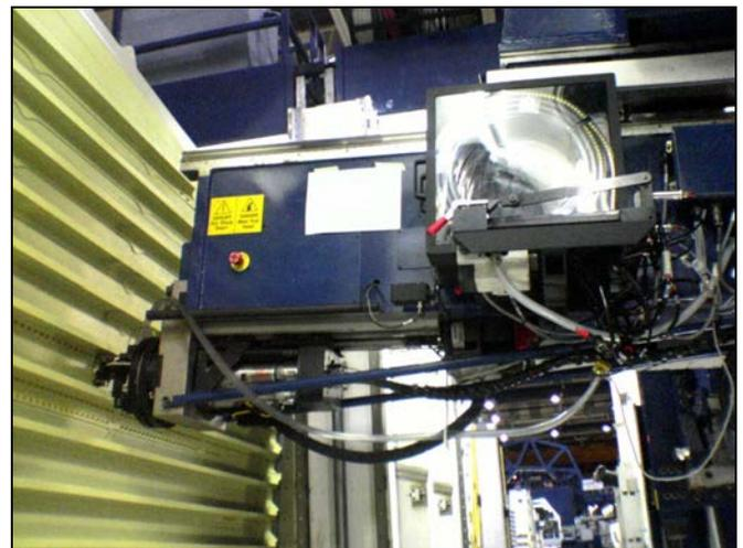
Figure 1 - Collar anvil and cartridge feed system
