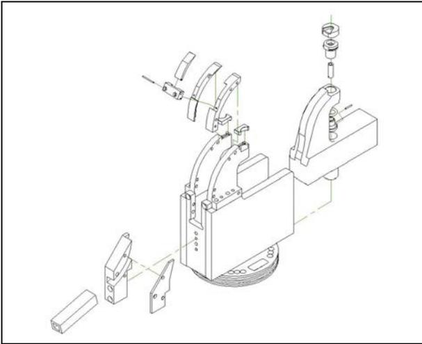
**Figure 3 - Exploded view of anvil and ram assemblies**
