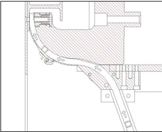
**Figure 7 - Step 3:** Ram is advanced to provide a specific clearance for the collar
