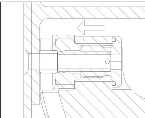
**Figure 9 - Step 5:** Ram moves toward work to capture collar against work piece in the bell-mouth of the die. Collar position and orientation verified via linear potentiometer
