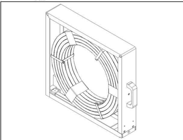
**Figure 4 - Collar cartridge assembly**
