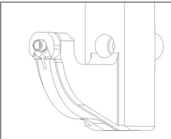
**Figure 8 - Step 4:** Collar is fed transverse through slot to sleeve. Sleeve has v-notch alignment feature to locate the collar
