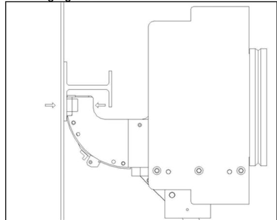
**Figure 5 - Step 1: Machine clamps up at a location**
