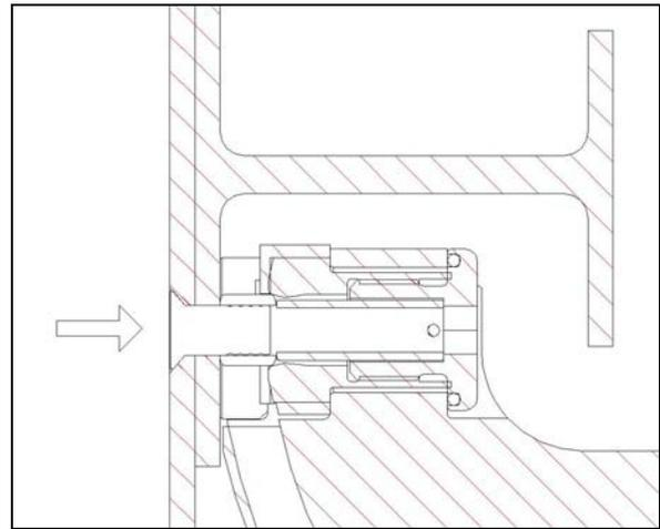
**Figure 10 - Step 6:** Bolt is driven through hole into collar. Tapered end of bolt aligns collar and die axis to bolt axis
