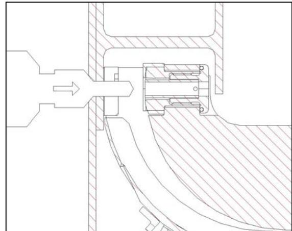
**Figure 6 - Step 2: Ram pulls back to allow drill breakthrough**
