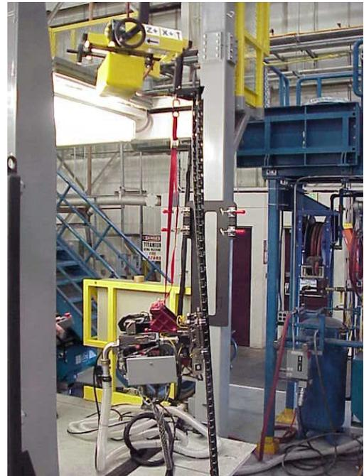
Figure 16: Vertical Handling with Adjustable Counterbalance
