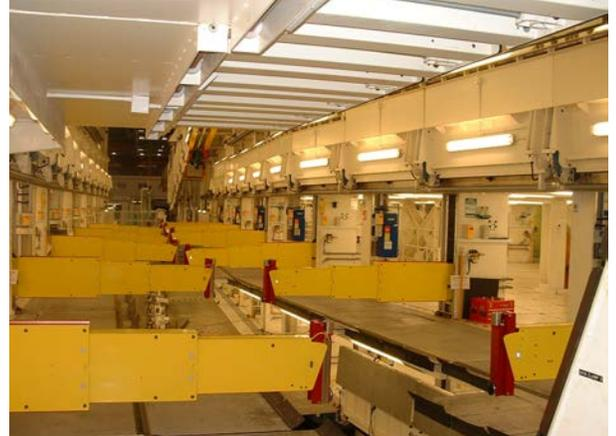
Figure 2, Eleven Panel Loader arms deployed on 2<sup>nd</sup> level empty starboard jig.
