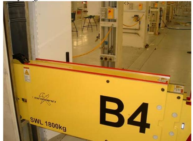
Figure 5, Arm deployed from Jig column, bumper strips top and bottom guard against crushing hazard.
