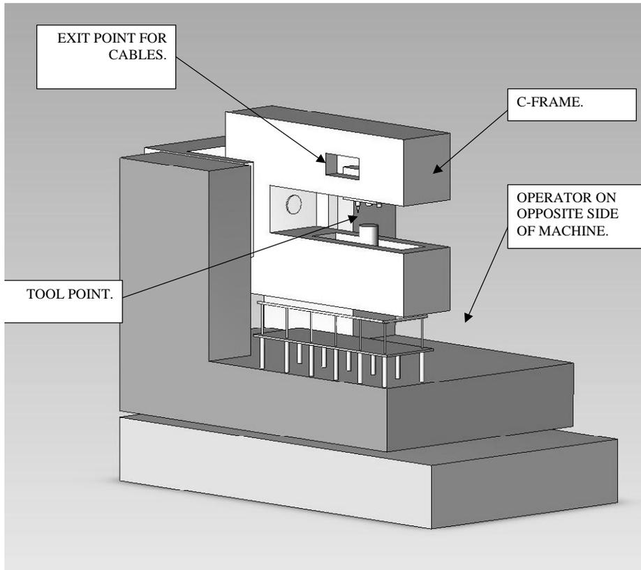
FIGURE 1: WING RIVETER.
