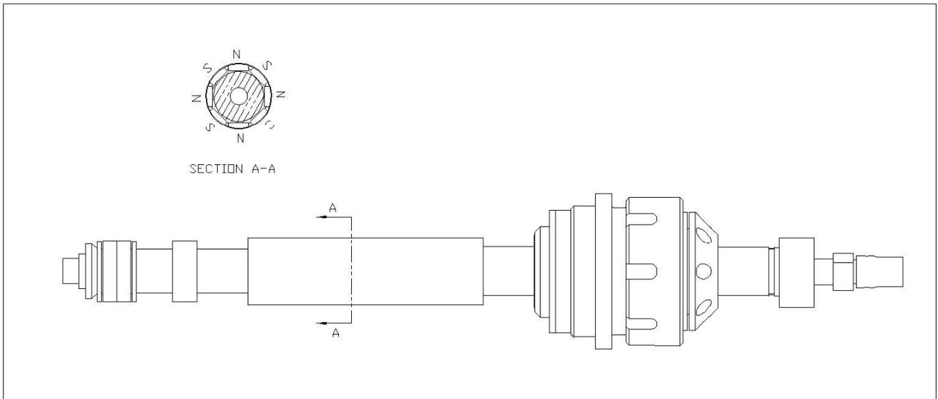
FIGURE 4: FOUR POLE PAIR MAGNET ROTOR
