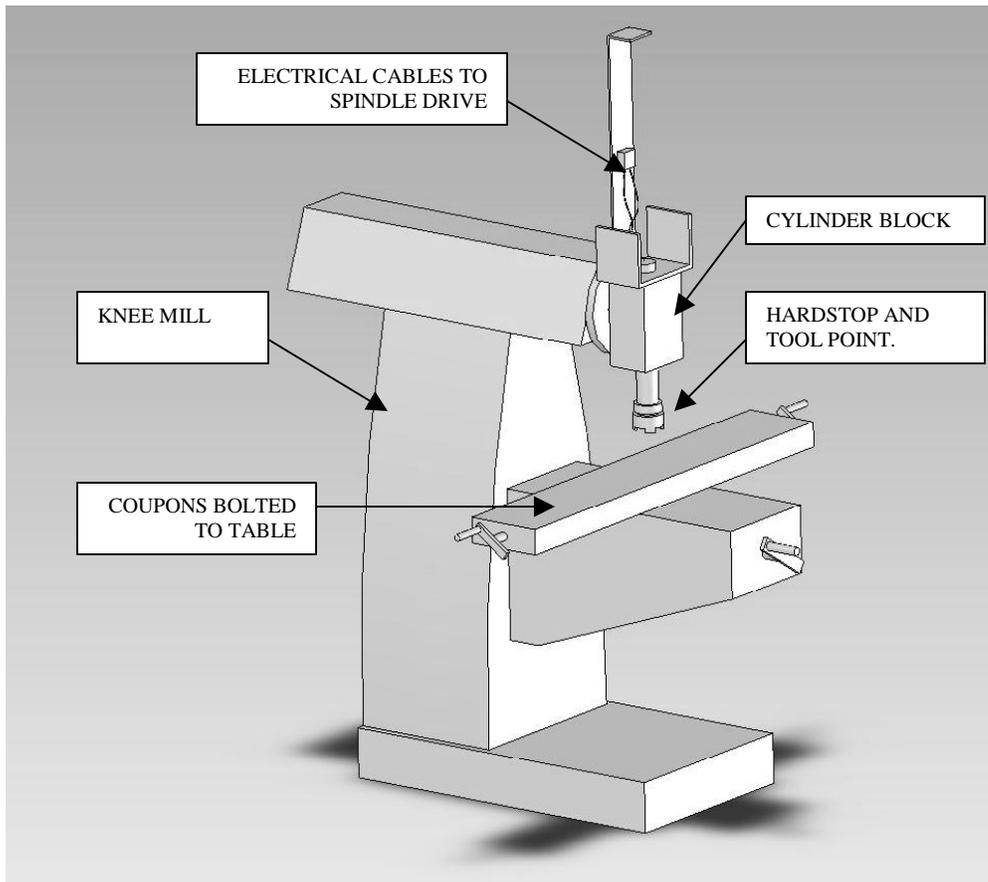
FIGURE 5: TEST SETUP FOR SPINDLE EVALUATION.
