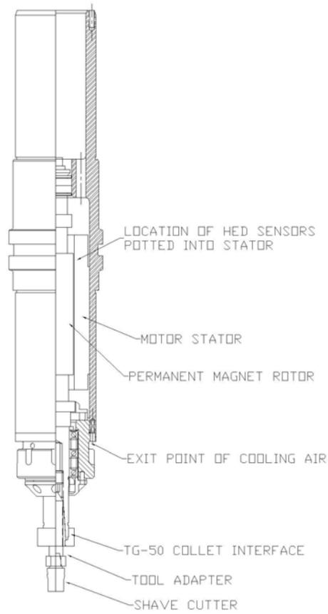
FIGURE 2: HIGH SPEED SHAVER ASSEMBLY DRAWING
