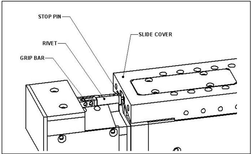
Figure 4: Diagram of the rivet chamber showing the rivet gripped between the stop pin and grip bar
