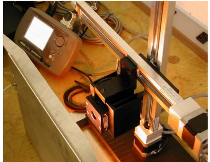
Figure 7 Power Meter on X/Y Stage Measuring Irradiance
