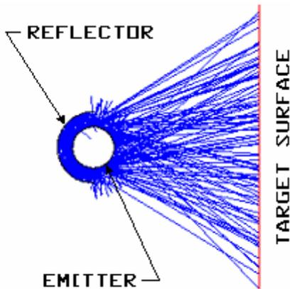
Figure 2. Ray-traced Model of IR lamp and reflector
