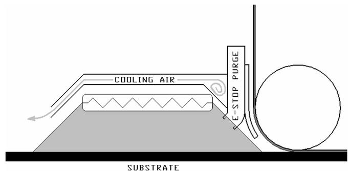
Figure 5. Secondary Heat Shield
