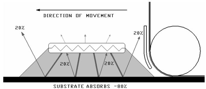
Figure 4. Undesirable Reflected IR and Waste Heat
