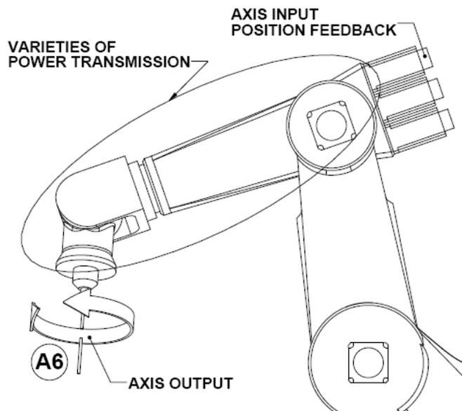
**Figure 2.** Standard location for position feedback
