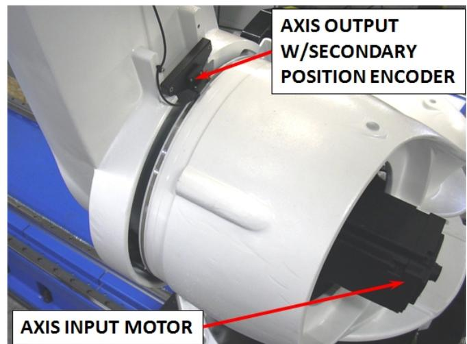
**Figure 4.** Applied secondary feedback at joint output
