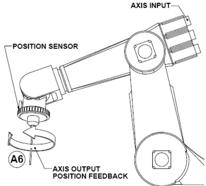
**Figure 3.** Secondary feedback at joint output
