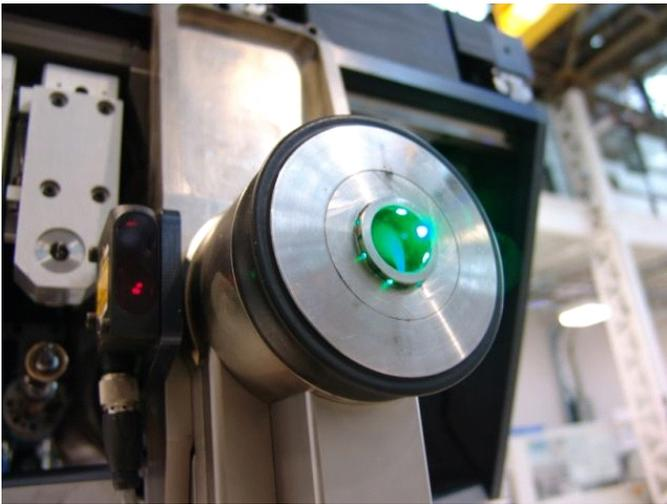
**Figure 7.** Auto-normalizing nose piece with integral flood coolant delivery with vacuum extraction
