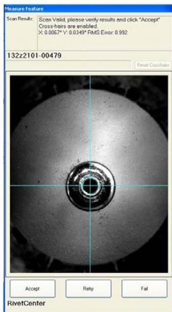
**Figure 6.** Image captured and recognized by automated vision system.
