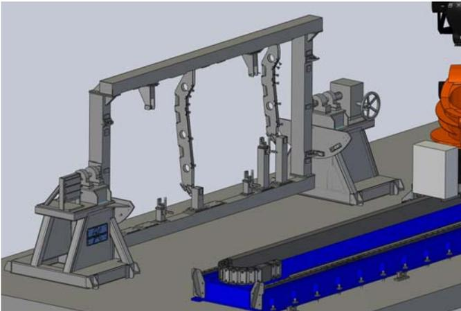
**Figure 1.** Rotating holding fixture
