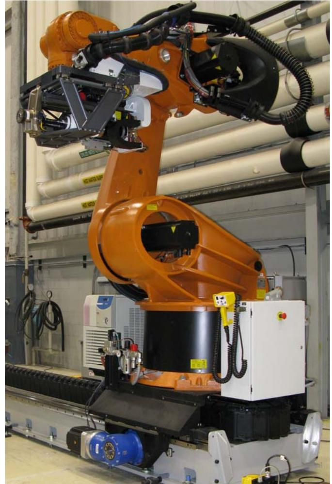
**Figure 2.** Positioning system - robot and track
