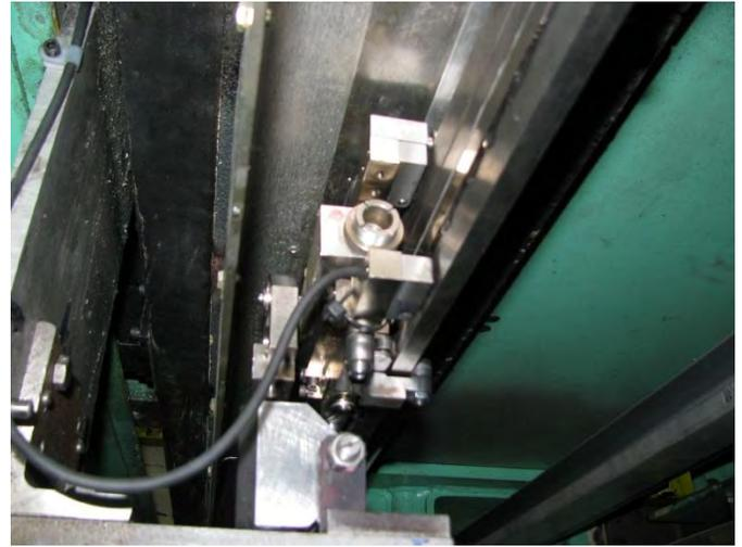
Figure 2: Installation of LM10 linear scale
