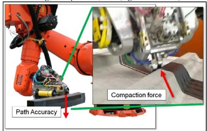
Figure 3. Robotic fiber placement
