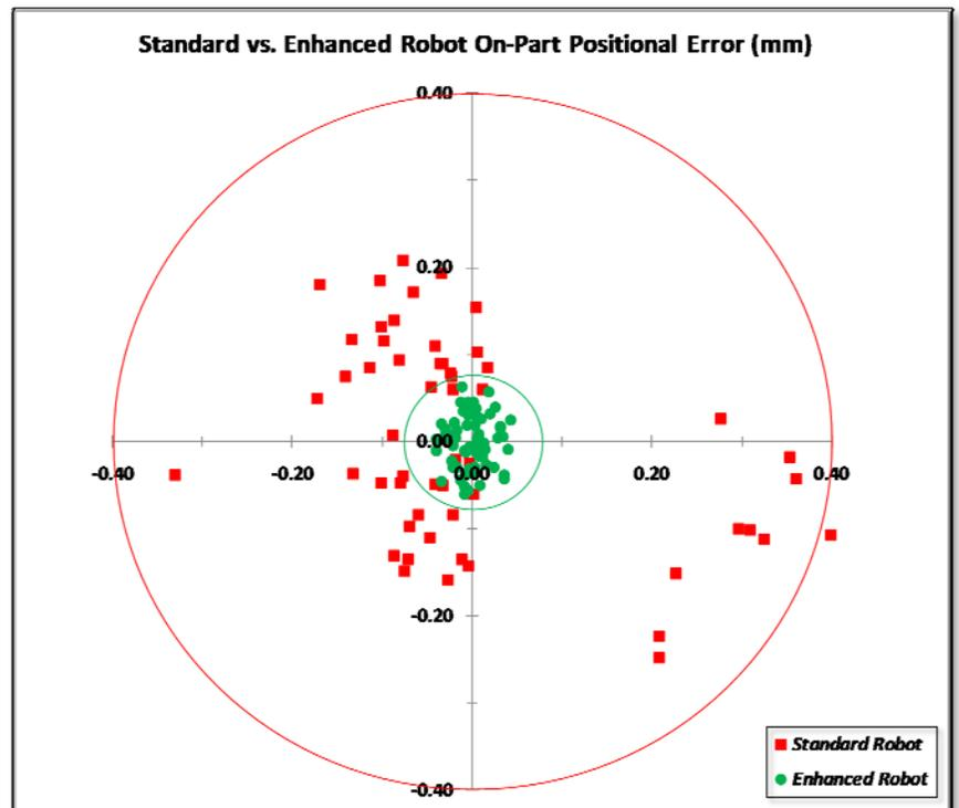
Figure 7. On-Part Accuracy Comparison
