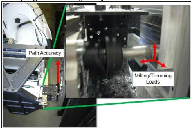
Figure 2. Robotic Milling/Trimming
