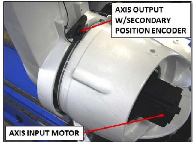
Figure 1. Robot axis with secondary encoder
