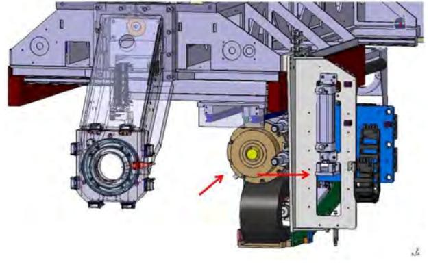
**Figure 8. First gripper retracts to clear spindle.**
