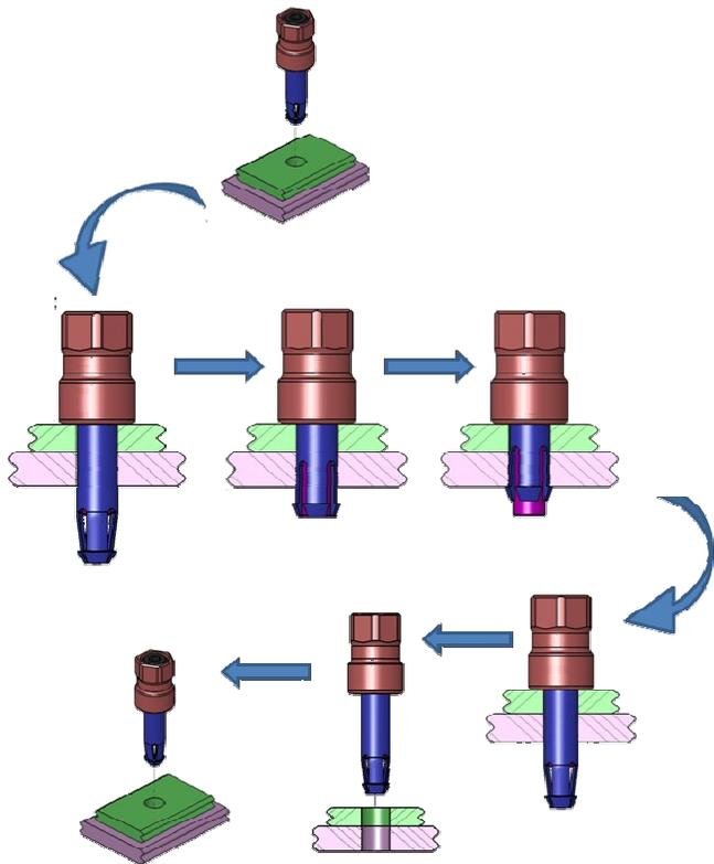
**Figure 2-SSTF Clamping and Unclamping**
