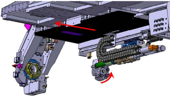
*Figure 10-Bolt Inserter Advances Revolver*
