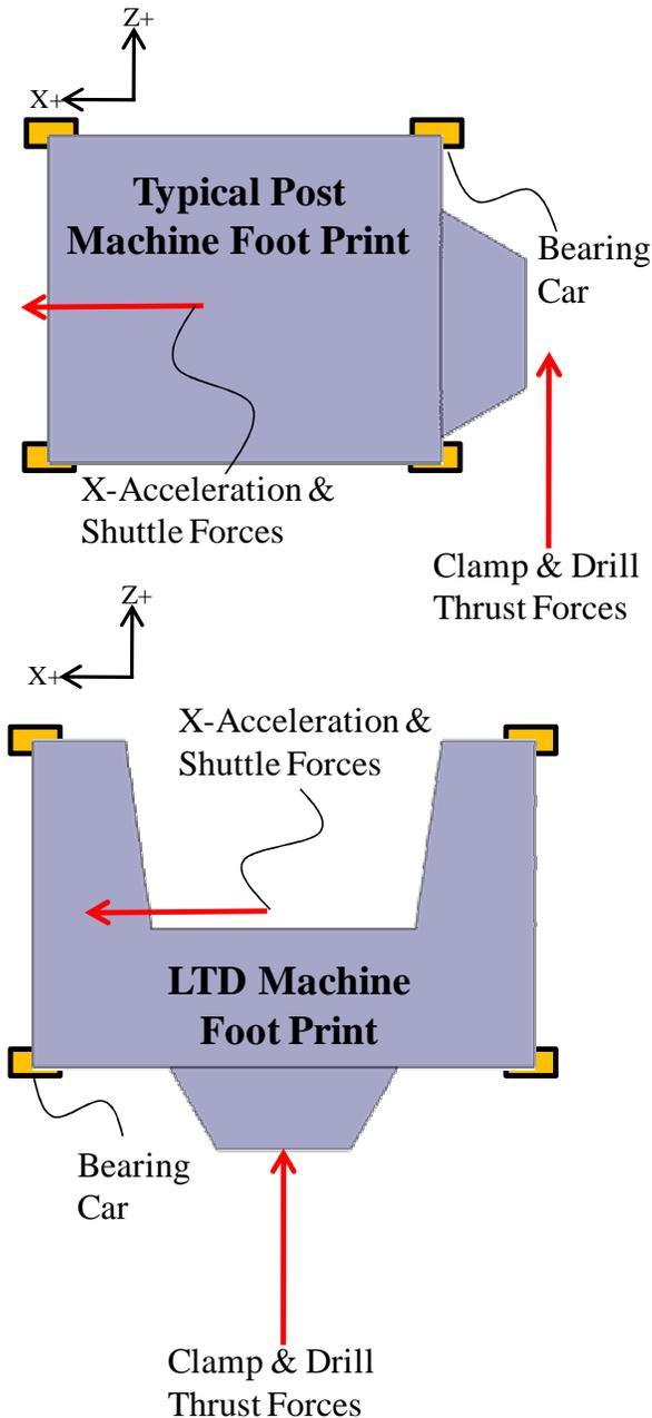
*Figure 5-Comparison of Acceleration and Thrust Force Vectors*
