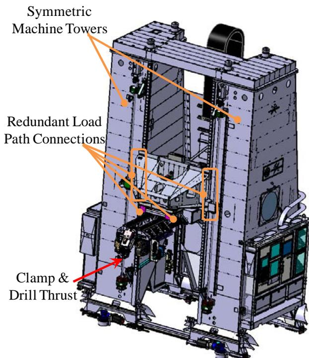
**Figure 4-Machine Load Paths**
