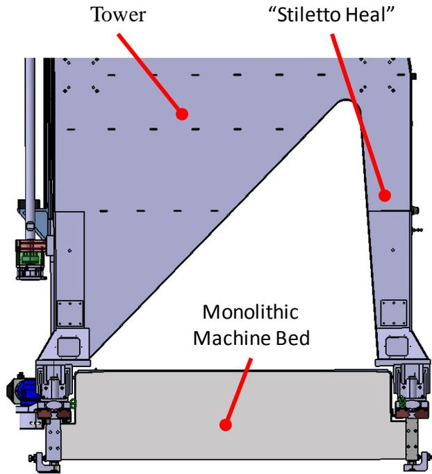
*Figure 6-Tower on Monolithic Machine Bed*
