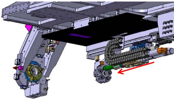
*Figure 9-Bolt Inserter Engages Fastener*
