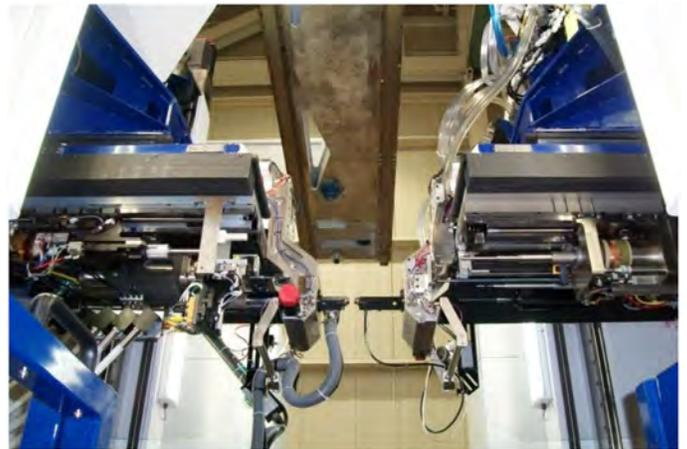
*Figure 3. Fastening heads of the ASAT2 machine.*
