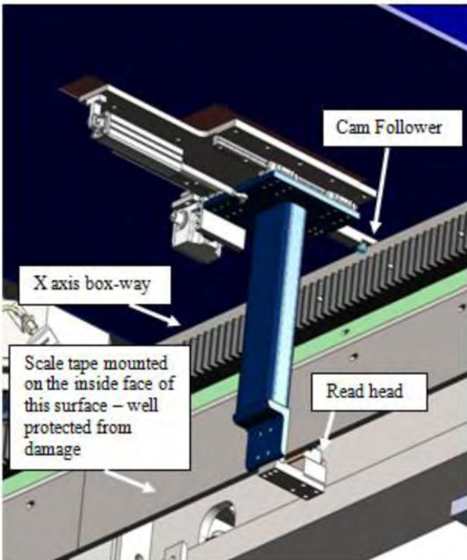
**Figure 7. Diagram showing the read head mounting, and rail follower.**
