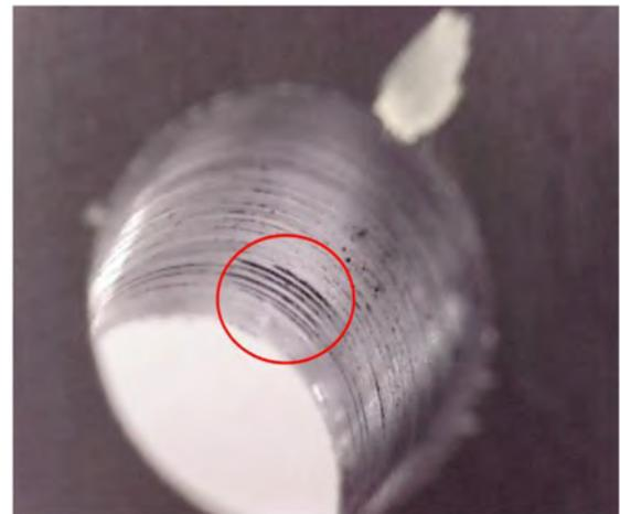
**Figure 12. Surface finish defects in under-sized drilled hole**
