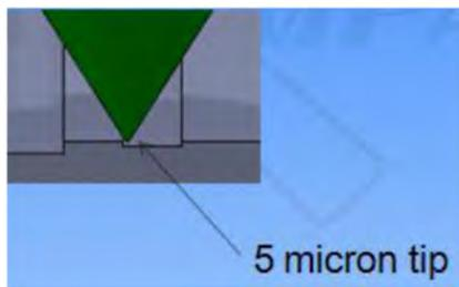
**Figure 2. Five micron probe tip shown with 0.25 mm ply thickness and 25 micron deep tear out.**
