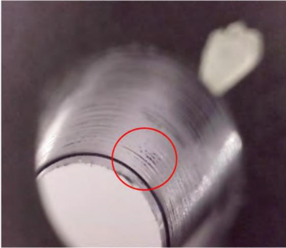
*Figure 13. Surface finish defects in reamed hole.*
