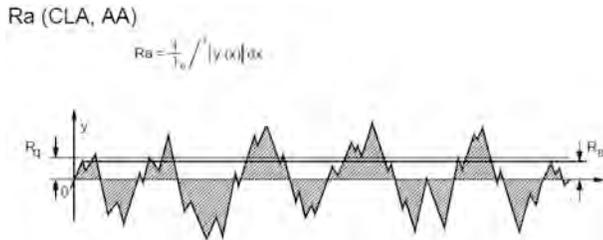
**Figure 1. Calculation of average surface roughness (Ra) per ISO 25178-2.**
