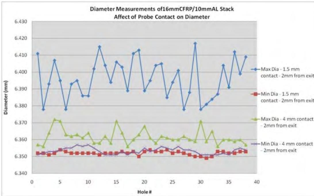
Figure 7. Hole probe diameter size effects.
