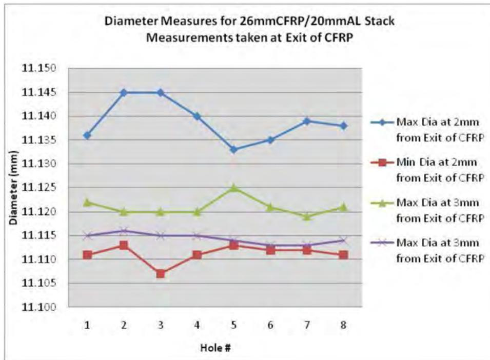
Figure 8. Axial location affects diameter measurements.
