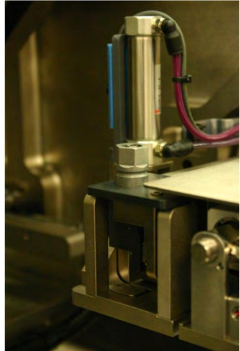
**Figure 9. Length check mechanism**
