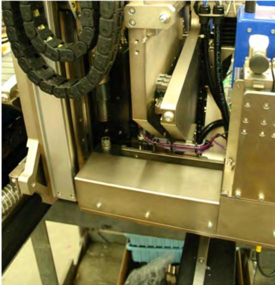
**Figure 7. Injector Cart extended placing bolt under Socket**
