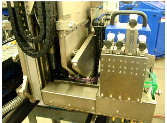
**Figure 6. Cartridge kicker is extended releasing a bolt**
