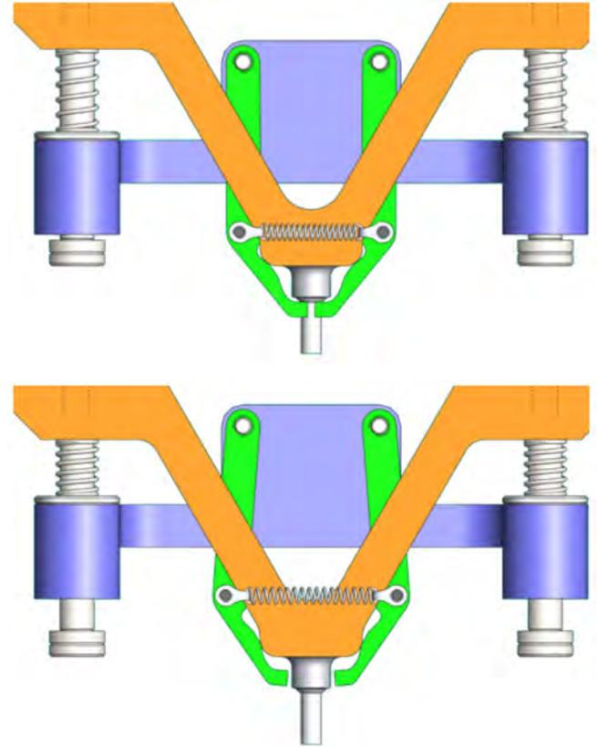
**Figure 8. Fingers releasing their grip on a rivet**
