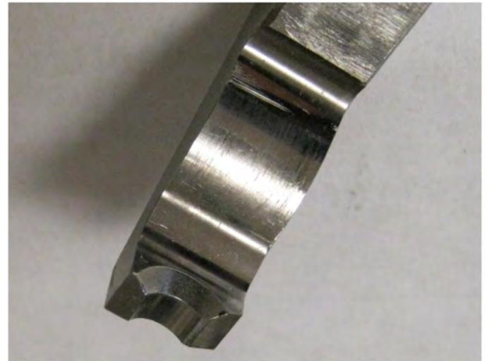
**Figure 9. NAS1097\*\*6 rivet finger tip detail**
