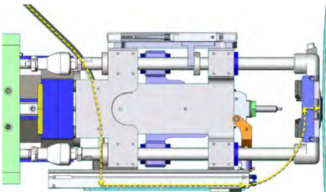
*Figure 11. Fastener feed path*
