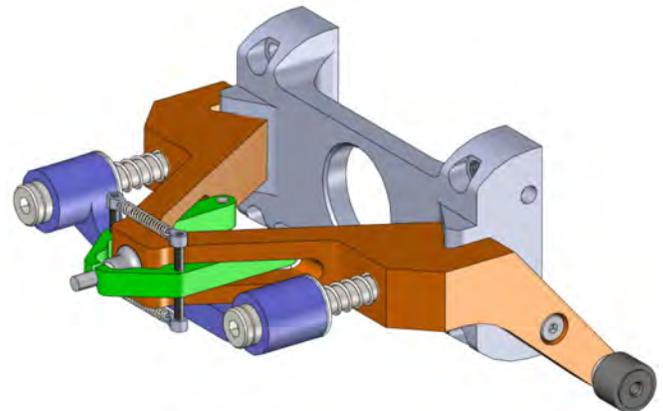
**Figure 6. Driver and pressure pad, ready to insert rivet (“drive” position)**
