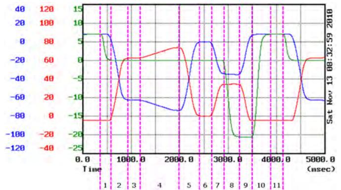
*Figure 13. Plot from CNC showing axis positions during a full cycle*
