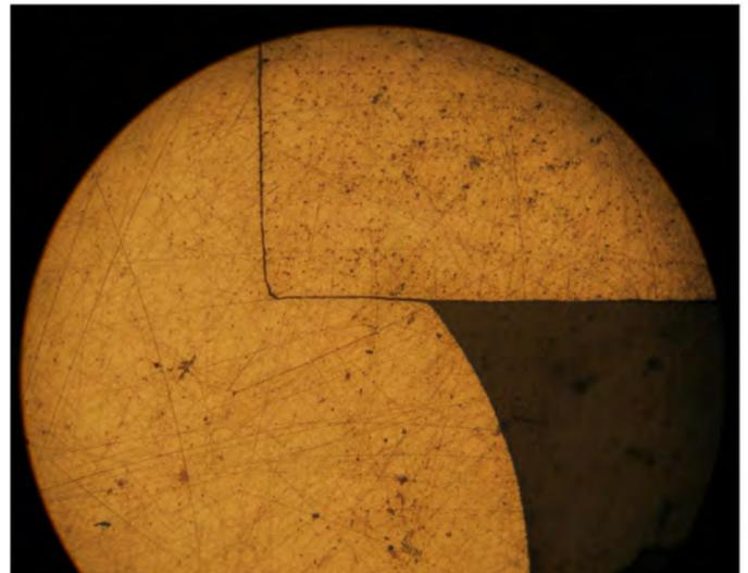
**Figure 15. Rivet tail (5x magnification)**
