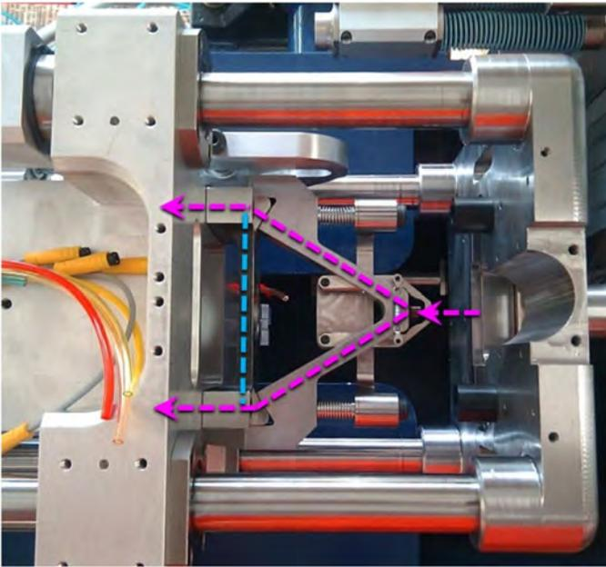
**Figure 7. Driver and pressure pad, showing areas of compressive (magenta) and tensile stress (blue) during rivet upset**
