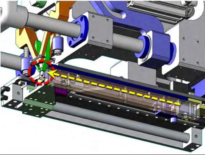
*Figure 10. Rivet injector showing feed path and rivet being snapped into fingers (circled)*
