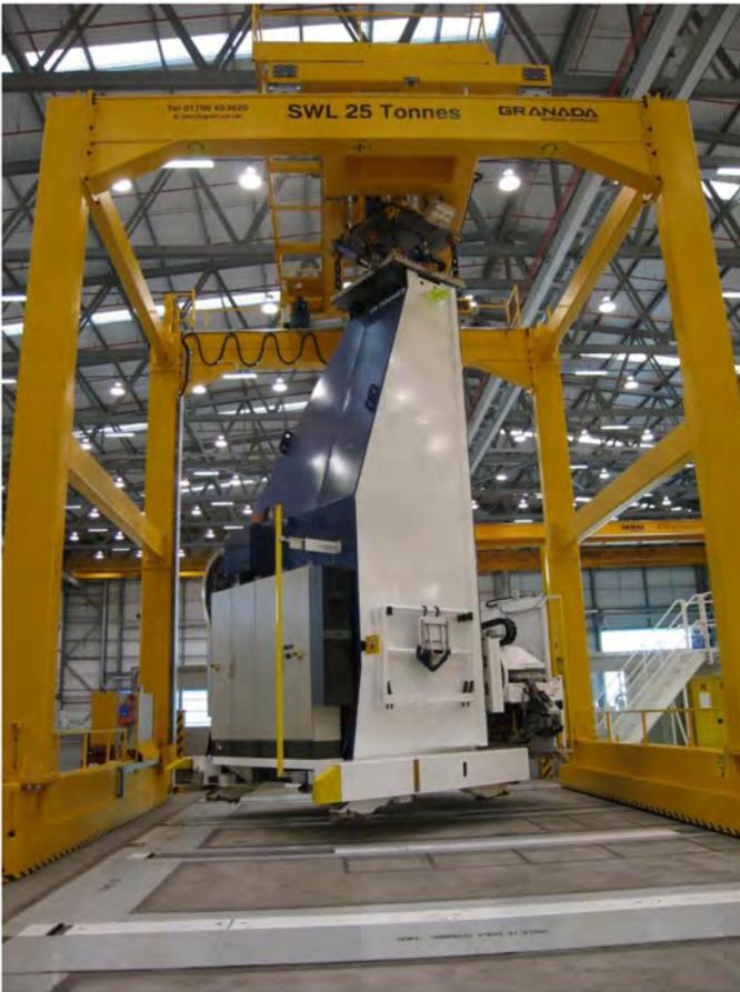
*Figure 2. This 5 axis moving column wing fastening machine has a working envelope far exceeding the operators reach.*
