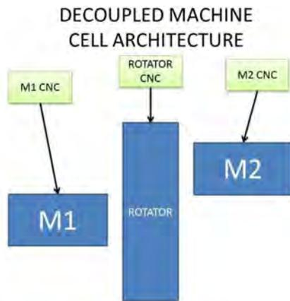
**Figure 6. Decoupled machine architecture, enabled by multiple technologies, including volumetric compensation.**
