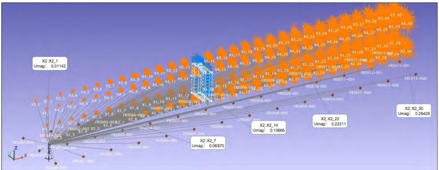
Figure 12. Uncertainty analysis of a single laser tracker station placed at the end of a 40m long cell. The increasing size of the uncertainty cloud reflects the magnitude and shape of the uncertainty measurements for that point.
