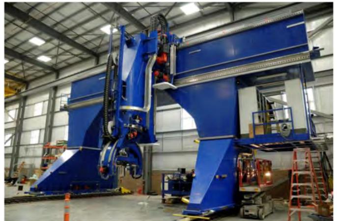
*Figure 3. Gantry style automated fiber placement machine with a large working envelope. The mass of such large machines may cause significant local foundation deflections that could affect the accuracy of a laser tracker placed nearby.*
