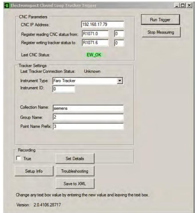
**Figure 10. This Electroimpact Closed Loop Tracker Trigger program facilitates two way Ethernet communication between a FANUC CNC and a tracker PC running Spatial Analyzer.**
