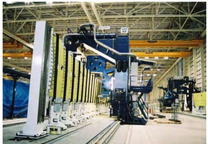
*Figure 1. This two tower, yoke style wing assembly machine requires 6 axis compensation and features unique geometries.*
