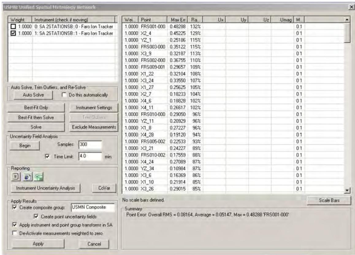
Figure 11. Running USMN Analysis in Spatial Analyzer.
