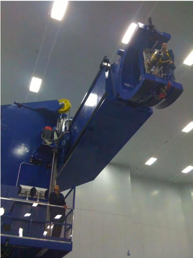
*Figure 8. There is no hope of an easy reach to the toolpoint on this moving column style automated fiber placement machine with its 6.4m (21') of vertical stroke. The Active Target becomes very useful when it is time to compensate this machine.*
