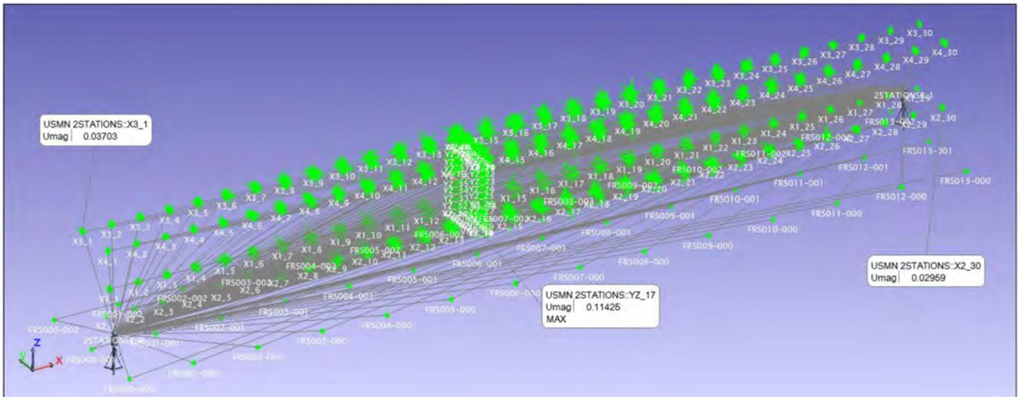
Figure 13. Uncertainty analysis of the previous cell, using a tracker station at each end of the cell. Error is now reasonable at both ends but unacceptable in the center.
