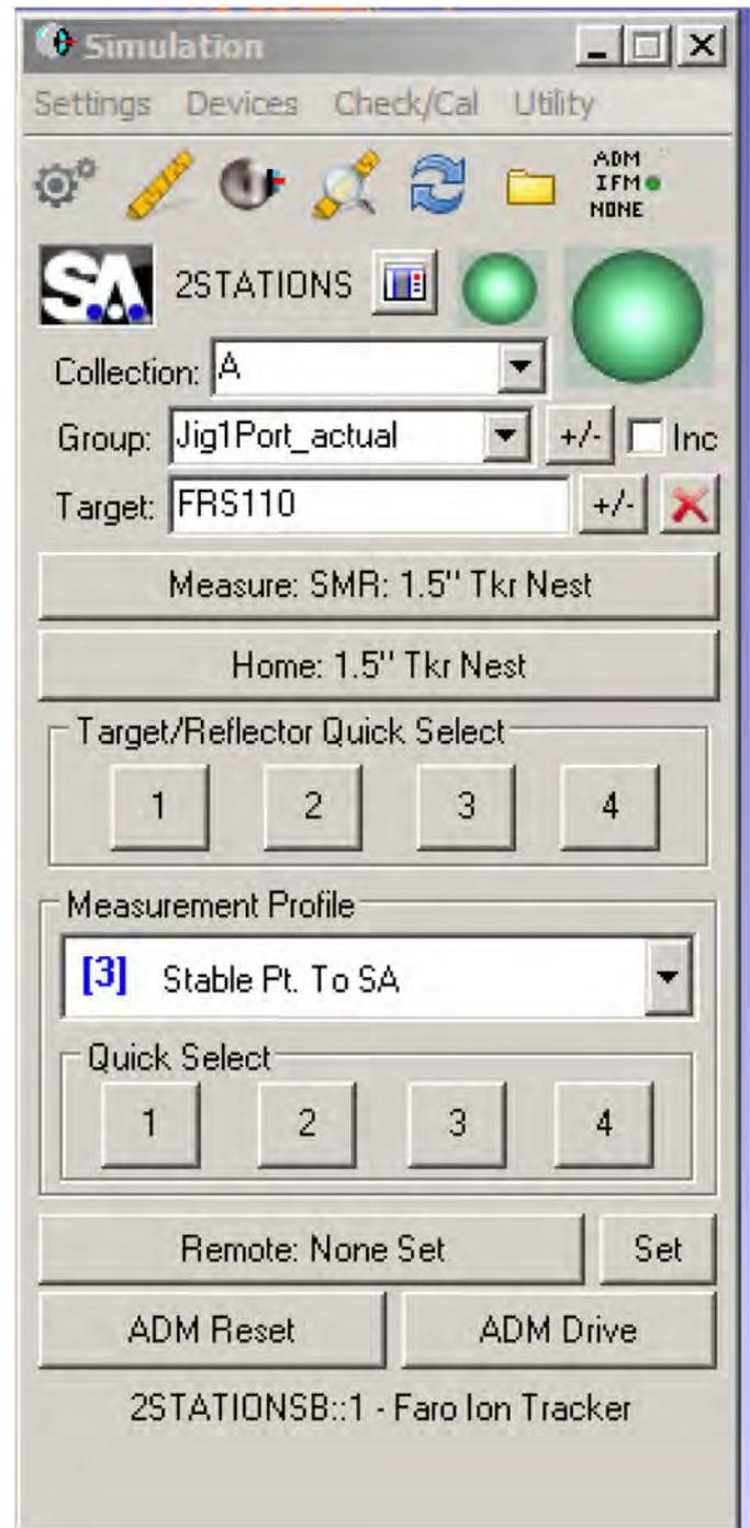
*Figure 9. The SA measurement window has a “Stable Pt To SA” tool that is especially useful for machine compensation.*
