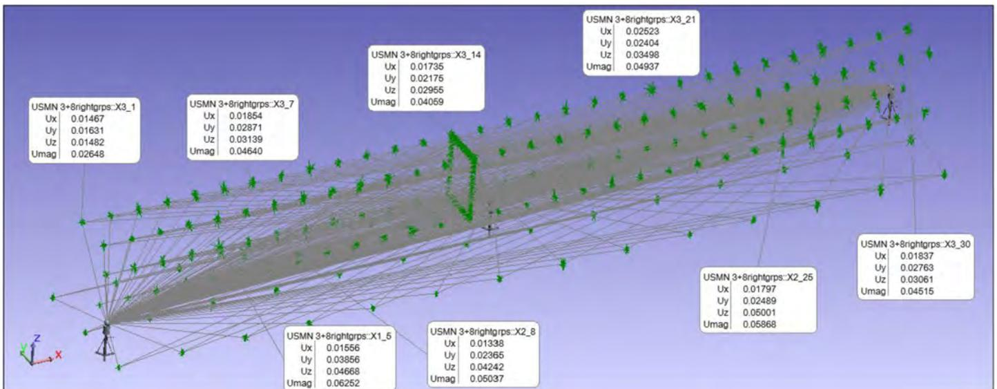
Figure 14. Uncertainty analysis of the previous cell, using 3 tracker stations. Uncertainty is now limited to about 0.07mm (.0028") throughout the working envelope.
