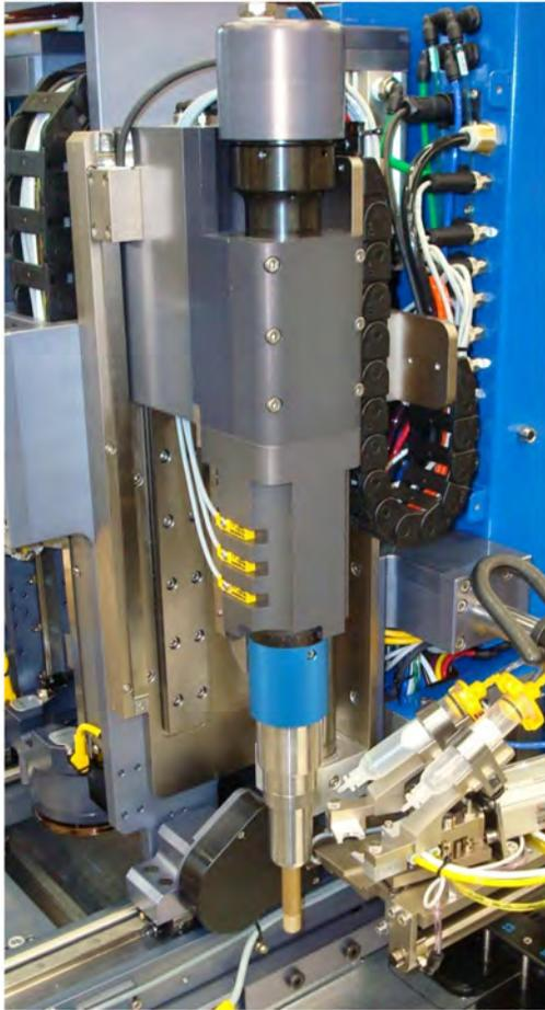
*Figure 4. Bolt inserter.*
