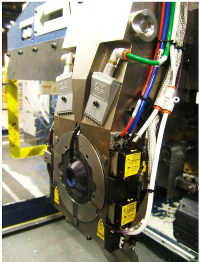
*Figure 6. Headstone with laser normality sensors*
