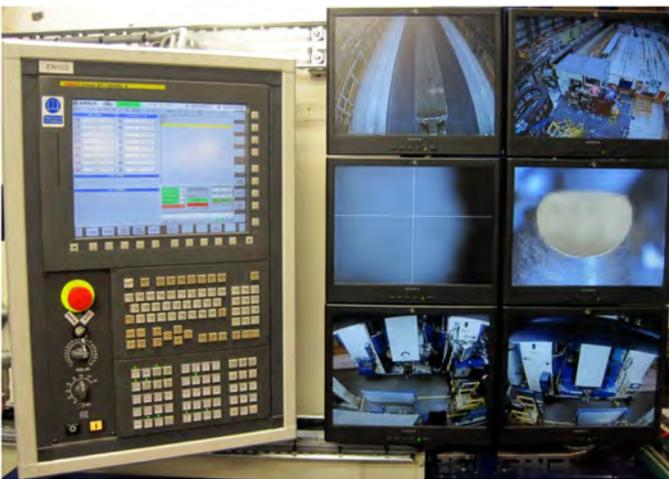
**Figure 3. 30i based operator interface**
