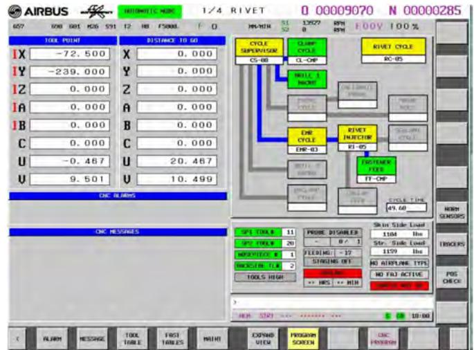
**Figure 4. 30i based custom HMI example screen**
