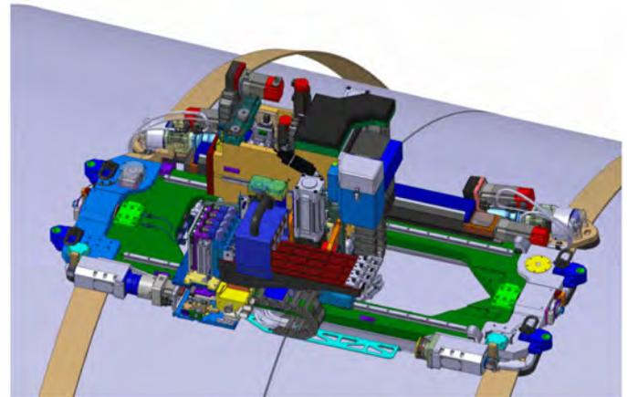
*Figure 1. 5-Axis Flex Track System*
